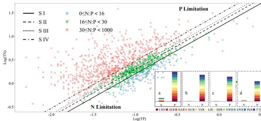
Fig. 4. TN and TP concentrations ( $\log_{10}$  transformed) from 1412 sampling sites (S I ~ S IV represents different criteria of nutritional limitation; the scatter shows the distribution of N:P under different criteria, the scatter on the top left of the line means P limitation, the scatter on the bottom right of the line means N limitation; a ~ d indicates the proportion of N limitation and P limitation under different criteria at each basin.)
