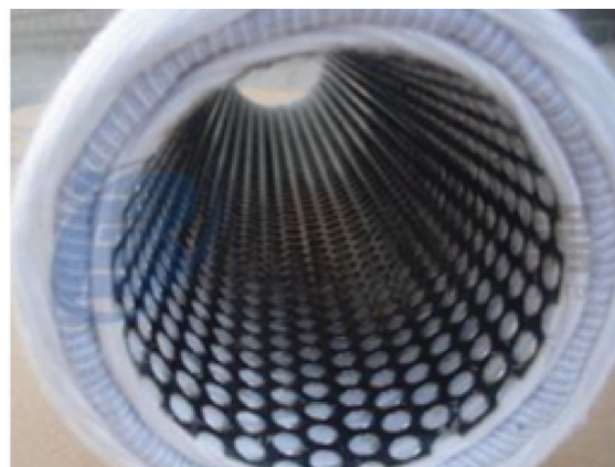
Fig. 5 Schematic of string-wound sediment cartridge filter. Suspended solids from untreated water will accumulate throughout the depth of the filter material, while dissolved contaminants are not retained. Therefore, the classification and removal efficacy of sediment filters is highly dependent on the pore size of the filter media (reprinted with permissions from 54,57 ; Copyright© Filters Fast LLC, 2020; Copyright© UNISUN, 2020).
