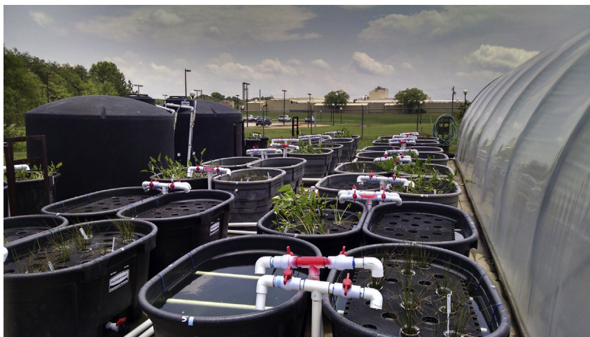
Fig. 1. Experimental layout showing thirty-two, 378.2 L mesocosms and two 5867 L stock tanks used to fill the mesocosms through water lines constructed using PVC piping and quarter turn valves.
