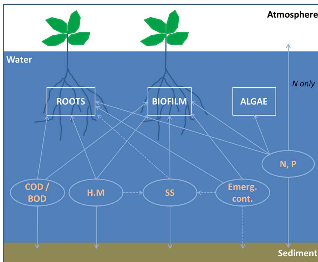
Fig. 1. Framework indicating the main removal pathways for key contaminant groups in the presence of CFWs. White squares indicate main compartments: ROOTS include uptake by the roots and the adsorption within the rhizosphere; BIOFILM indicates the microbial degradation within the rhizosphere; ALGAE describes the uptake by phytoplankton. Dashed line indicates adsorption only; Emerg. cont. = emerging contaminants (i.e. herbicides, pesticides, PPCPs), H.M. = heavy metals.
