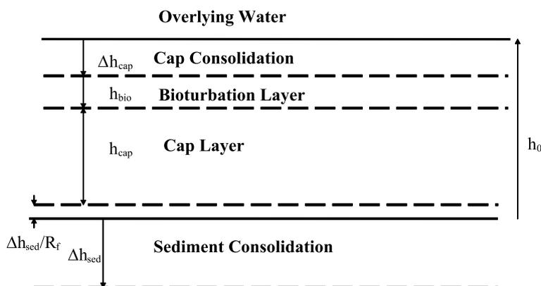
**Fig. 1** Conceptual model of a sediment cap
