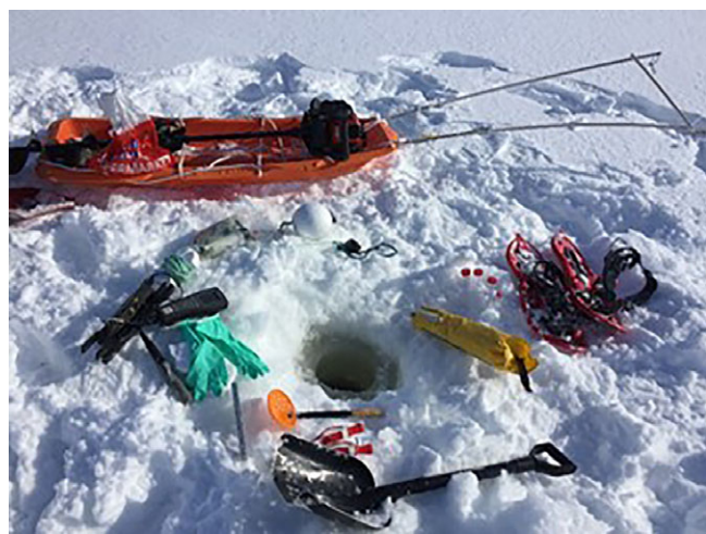
Fig. 2. Examples of winter field equipment: pulka, motorized ice auger, sieve, shovel, snowshoes, and safety rope.
