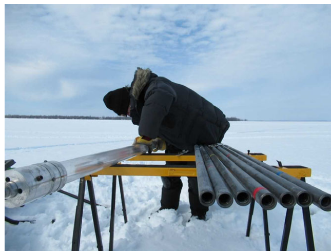
Fig. 1. Example of coring setup on the ice. Elevated stands keep equipment out of the snow and ice and can help prevent equipment from freezing.
