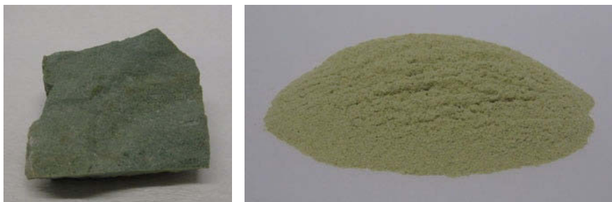
Fig. 1. The rock sample of HENZA (left) and the grain-size <0.5 mm of HENZA (right), used in the butch-type experiments.
