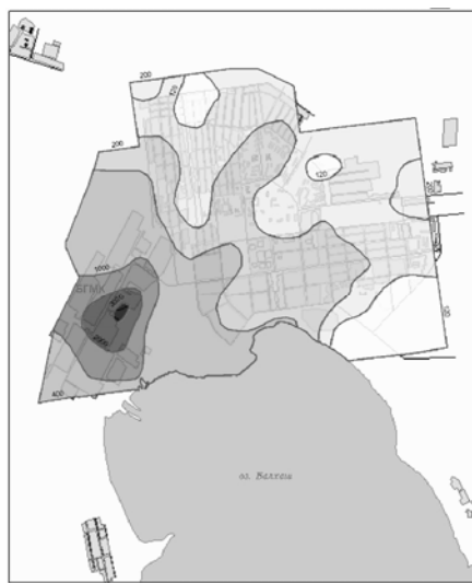
Figure 3. Pollution of the soil surface layer. total zinc in Balkhash city in 1992. Reference: Pollution in the units of background C_f = 25 \text{ mg/kg} . Range of variation from 120 to more than 200
